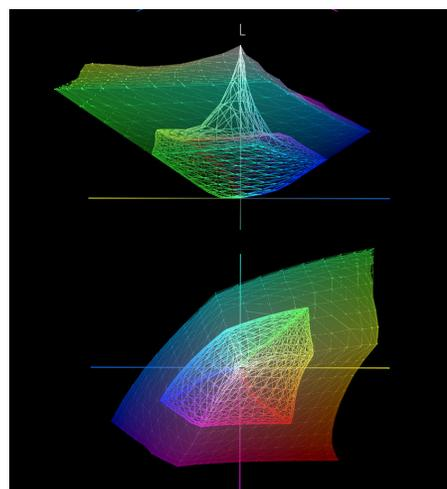
Sample gamut volume of an RGBW 1DLP projector w/.32 color luminance ratio. Presentation Mode (transparent solid) vs. sRGB mode (wireframe.)
