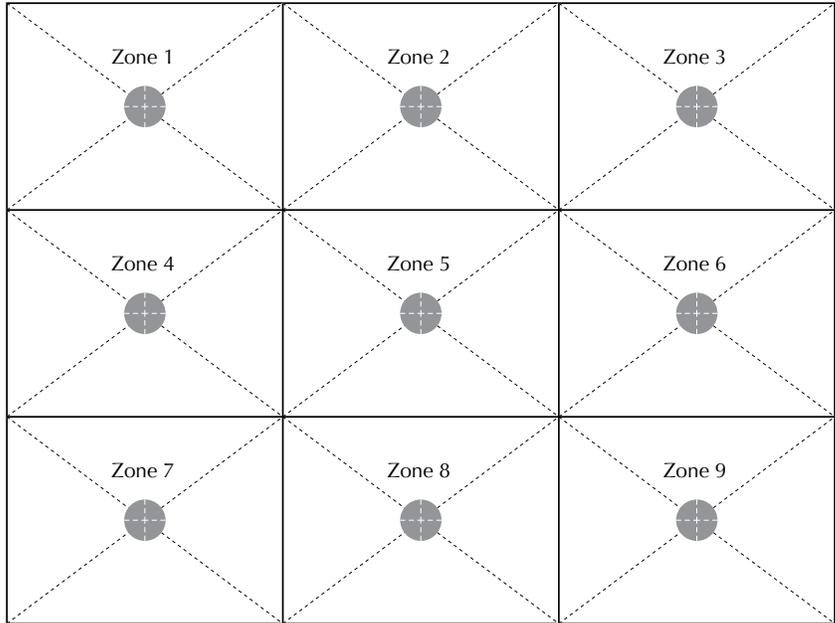
Figure A.7 - 9 point measurement grid for illuminance testing.
