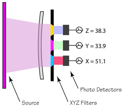
The **XYZ Colorimeter** is very simple and inexpensive. It has three detectors one each for X,Y and Z. These detectors are much larger and therefore have much better signal-to-noise ratios. The direct result is X,Y,Z data of high accuracy. The large sensors mean that low light levels produce a stronger signal. Because, the light from each sensor is from many spectral bands not just one, the total energy is even greater creating even better signal-to-noise ratios.
