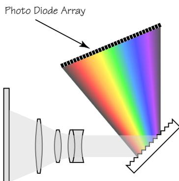
**Lower cost spectroradiometers** use an array of photodetectors (usually photodiodes.) These detectors do not have the signal-to-noise ratio of the photomultiplier in the lab grade unit. The array also has gaps between each detector. The device can't see a change in the spectrum near these gaps.
