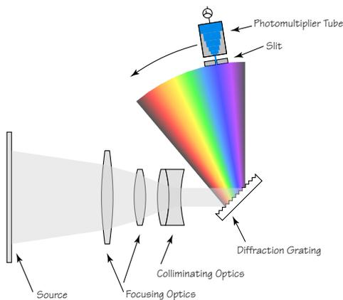
The **Lab Grade Spectroradiometer** is very expensive, slow, and very accurate.
