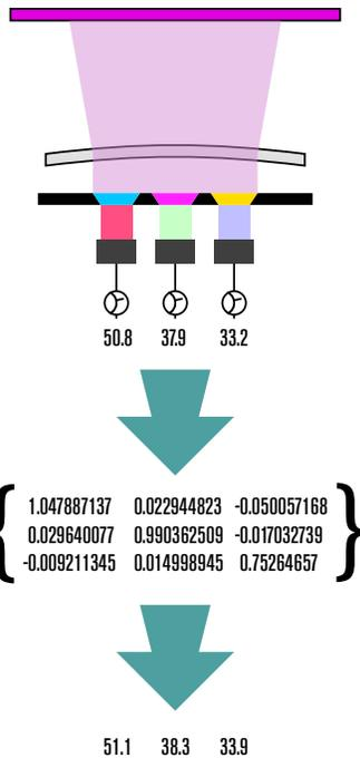
When a colorimeter is calibrated to the source primaries of a display with a calibration matrix. The accuracy of the colorimeter on that type of display is greatly increased. The worst case accuracy of this type of purpose built colorimeter can not be matched with a spectroradiometer anywhere near the price. In fact you would have to spend 100 times as much to achieve this accuracy with a spectroradiometer.
